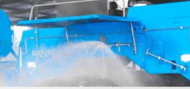
Process optimization injecting water during turning
