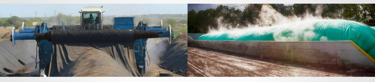
The best synergy: a combination of windrow turner with integrated cover winder and the membrane covered system.
