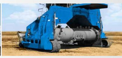
For increased traction on loose ground the landfill undercarriage
