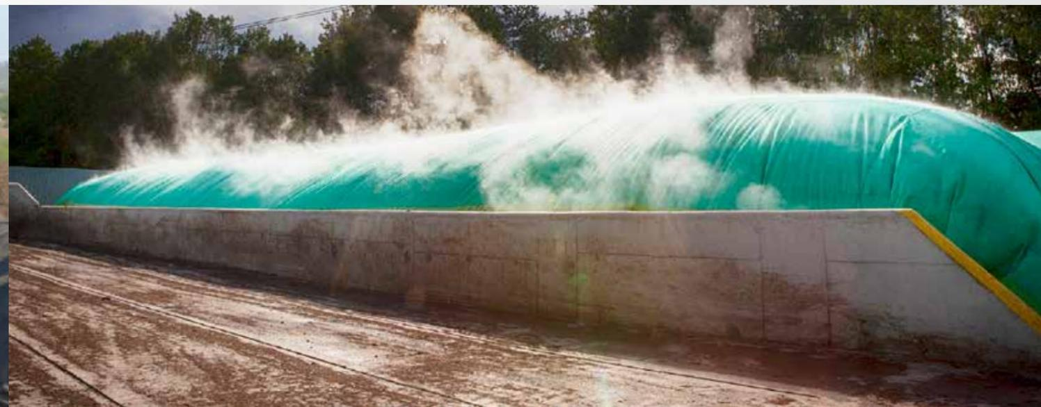
The best synergy: a combination of windrow turner with integrated cover winder and the membrane covered system.
