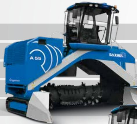
length 5,100, width 5,700, height 4,650, rotor diameter 1,200
