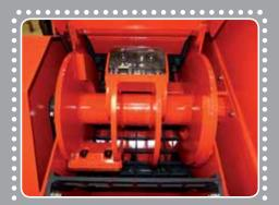
The rotor with a diameter of 600 mm and 6 blades has a huge flywheel
